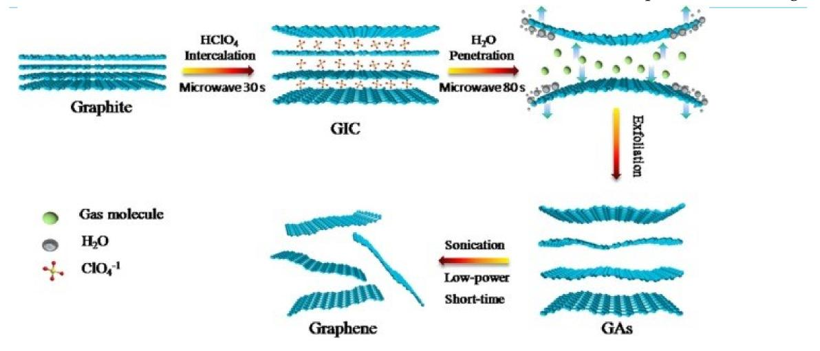
Chemical exfoliation is a top-down approach to obtain graphene in dispersion from graphite using stages of intercalation, exfoliation, and sonification The advantage of this manufacturing route is that the intercalation compounds spontaneously dissolve in polar solvents.
