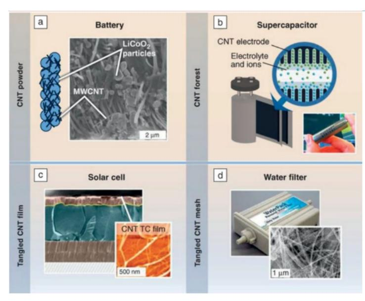
Energy-related applications of nanotubes. (a) Mixture of multiwall carbon nanotubes (MWCNTs) and electrochemically active powder for a battery electrode. (b) Concept for supercapacitors based on CNT forests. (c) Solar cell using a single-wall-carbonnanotube-based transparent conductor (TC) film. (d) Prototype portable water filter using a functionalized tangled CNT mesh in the latest stage of development..
