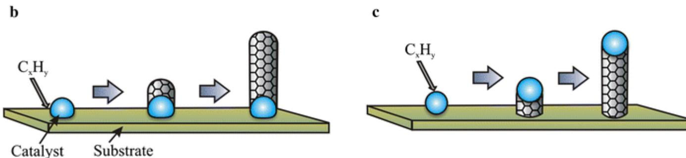
Hydrocarbon gas + Fe/Co/Ni catalyst at 550-1000°C
