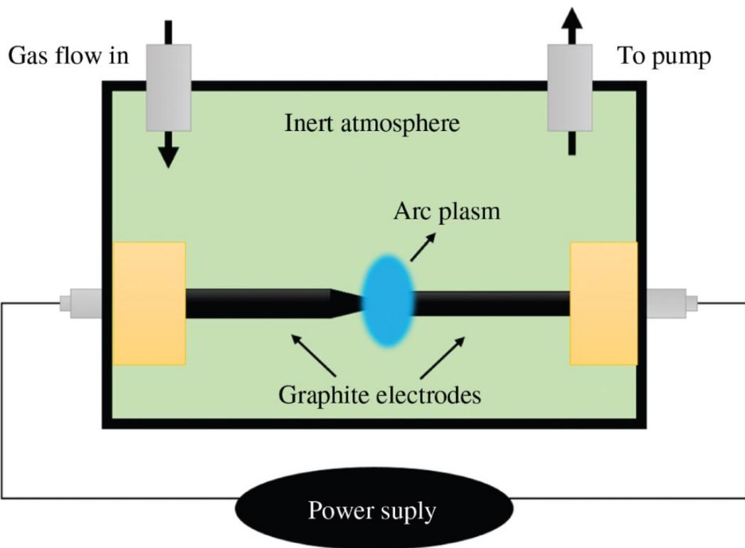
*Electric arc discharge method* for the production of fullerenes is based on the evaporation of graphite electrodes in a low-pressure helium atmosphere by passing an electrical current through the electrodes, resulting in an arc that produces carbon black containing fullerenes.
