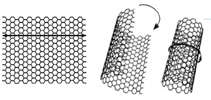
CNT is configurationally equivalent to a two-dimensional graphene sheet rolled into a tube.
