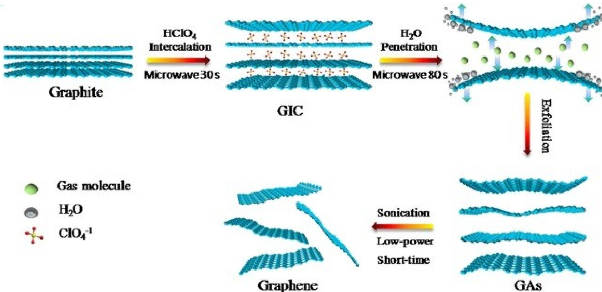
Chemical exfoliation is a top-down approach to obtain graphene in dispersion from graphite using stages of intercalation, exfoliation, and sonification. The advantage of this manufacturing route is that the intercalation compounds spontaneously dissolve in polar solvents.
