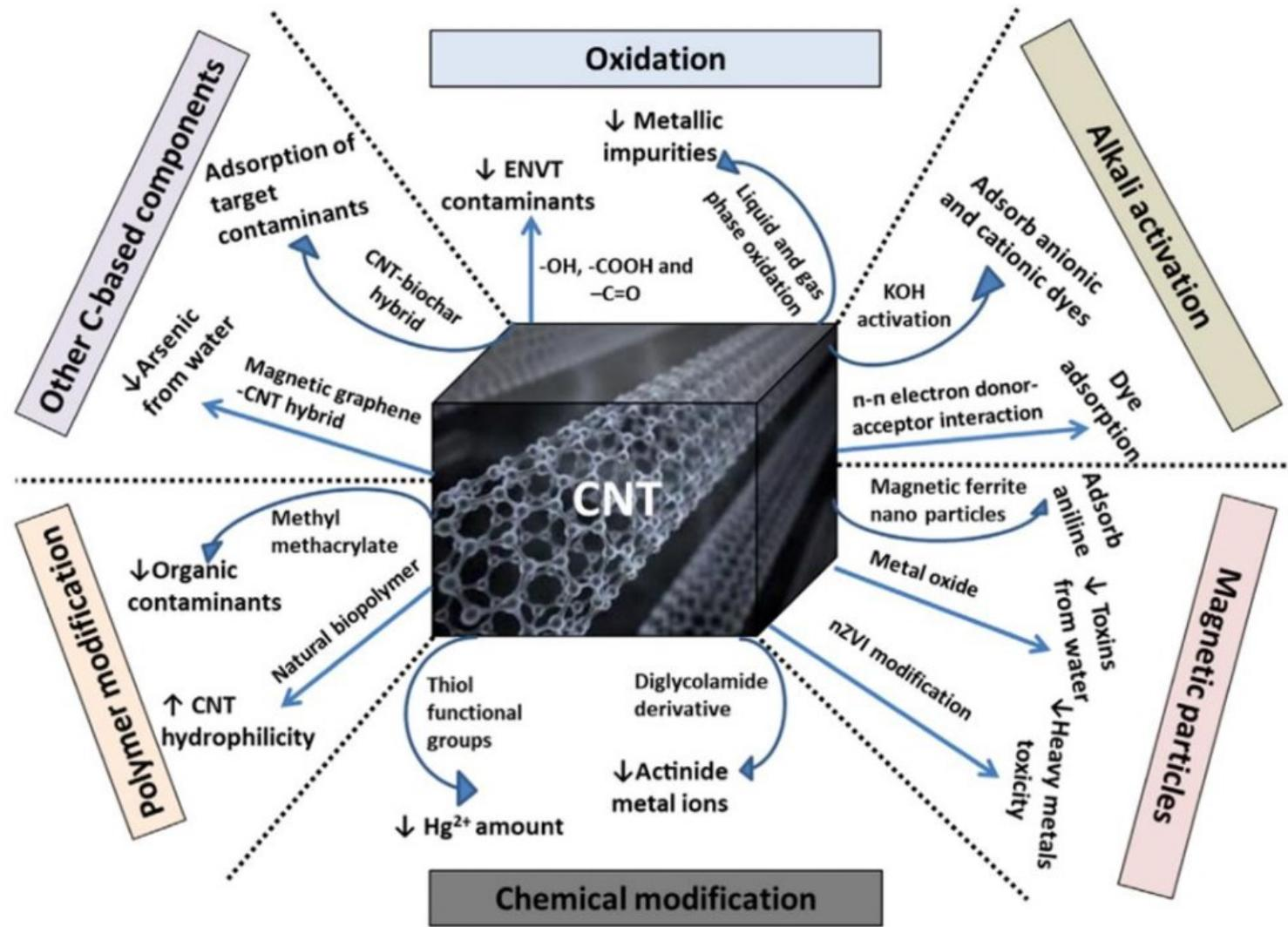
Schematic diagram representing different modification processes of CNTs for contaminant removal from water and wastewater (C: carbon; CNT: carbon nanotube; ENVt: environmental; Hg: mercury; KOH: potassium hydroxide)
