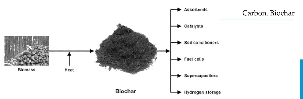
Biochar is produced by burning organic material in a controlled pyrolysis (burning without oxygen). The energy or heat generated during pyrolysis can be collected and used as clean energy. Biochar is much more efficient at converting carbon into a stable form and cleaner than other forms of charcoal.
