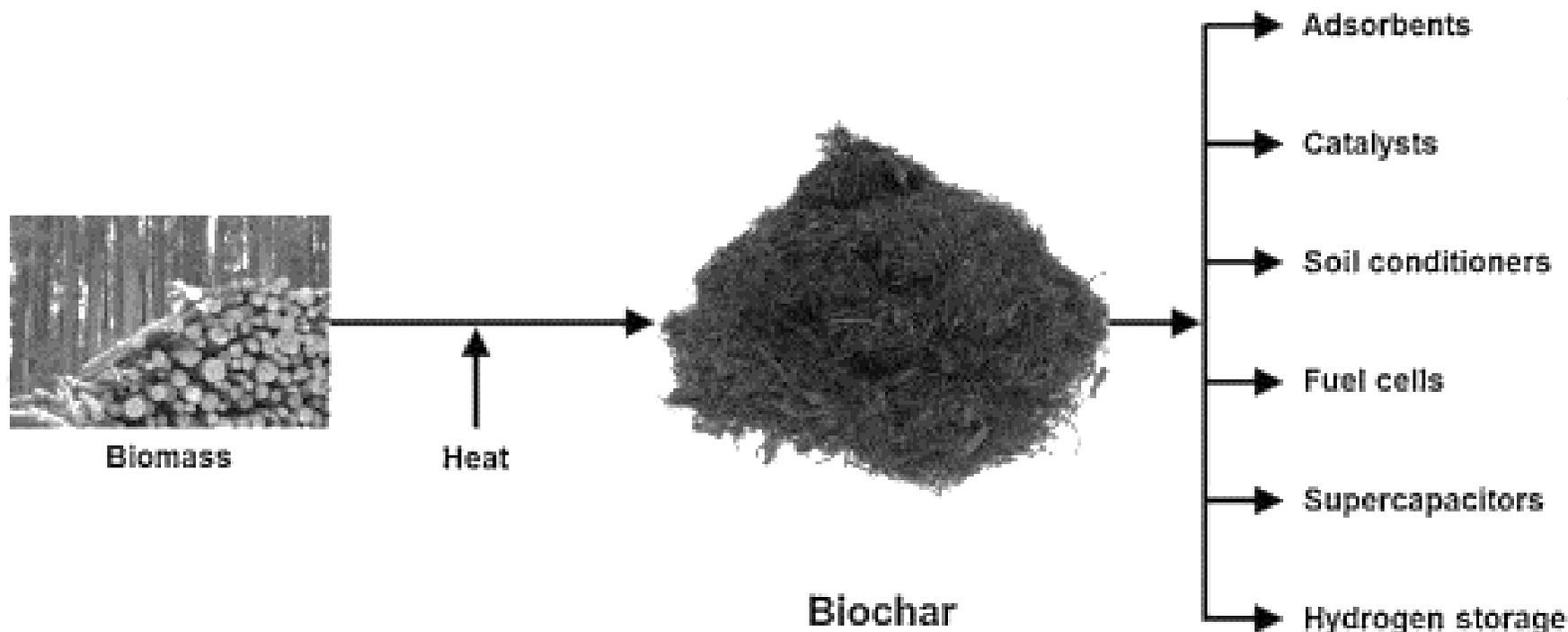
Biochar is produced by burning organic material in a controlled pyrolysis (burning without oxygen). The energy or heat generated during pyrolysis can be collected and used as clean energy. Biochar is much more efficient at converting carbon into a stable form and cleaner than other forms of charcoal.
