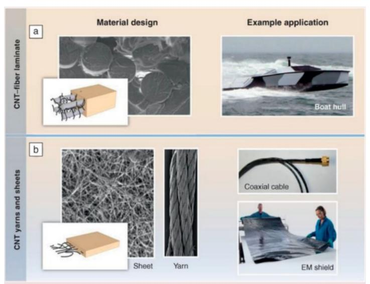
Nanotube composites and macrostructures. (a) Micrograph showing the cross section of a carbon-fi ber laminate with carbon nanotubes (CNTs) dispersed in the epoxy resin and photograph of a lightweight CNT-fi ber composite boat hull for maritime security boats. (b) Micrographs of CNT sheet and yarn, and photographs of their use in lightweight data cables and electromagnetic (EM) shielding material.
