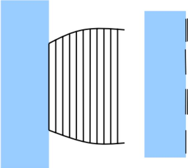
In *micromechanical exfoliation method*, graphene is separated from a graphite crystal using adhesive tape. After peeling it off the graphite, multiple-layer graphene remains on the tape. By repeated peeling the multiple-layer graphene is cleaved into several flakes of few-layer graphene.
