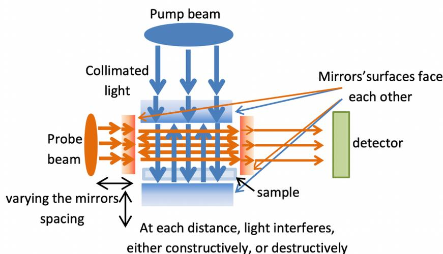
Fig. 1. Geometry of the upgraded PTD system with a resonant cavity
