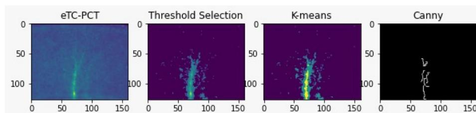
**Fig. 2:** eTC-PCT images of a surface-terminating crack in a steel sample. The raw eTC-PCT images of the crack are presented before processing and after threshold selection (step 1), K-means clustering (step 2); and the final canny edge detection (step 3). The result is a crack image reconstruction with sharply delineated boundaries.
