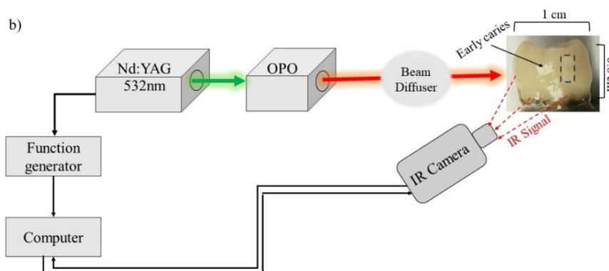
**Fig. 3.** Experimental configuration of multispectral eTC-PCT system and photograph of a tooth sample with early caries.
