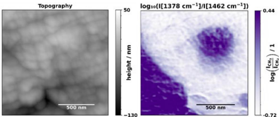
**Fig. 3.** Topography and band ratio of the bands corresponding to deformation vibrations of  $\text{CH}_2$  and symmetric deformation of  $\text{CH}_3$  groups ( $1.5 \mu\text{m} \times 1.5 \mu\text{m}$ ).
