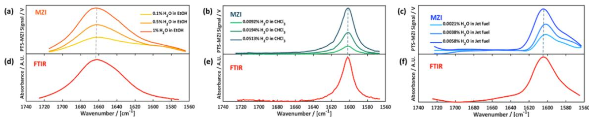
**Fig. 2.** PTS spectra of the water bending vibration as recorded using the Mach Zehnder Interferometer (MZI) and compared to the those recorded on a standard FTIR spectrometer. **(a),(d)**: water in ethanol, **(b),(e)** water in chloroform and **(c),(f)** water in jet-fuel. The differences in the spectral shape result from different H-bonding of the water molecule in the studies solvents and solvent system (jet-fuel).
