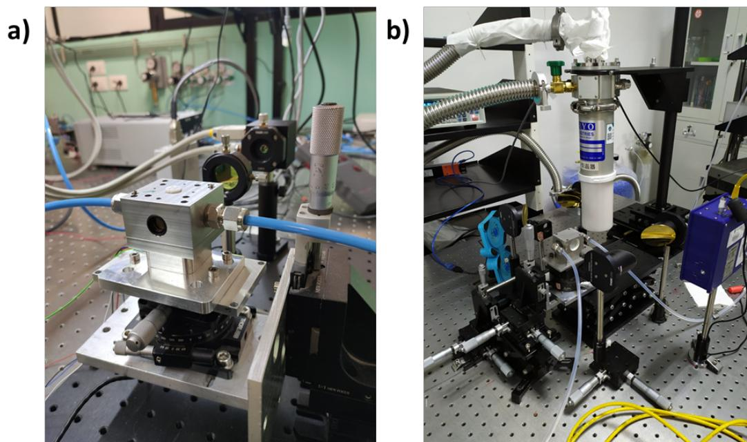
**Fig. 1.** Picture of the near-IR H<sub>2</sub>S QEPAS sensor (a) and of the THz H<sub>2</sub>S QEPAS sensor (b).
