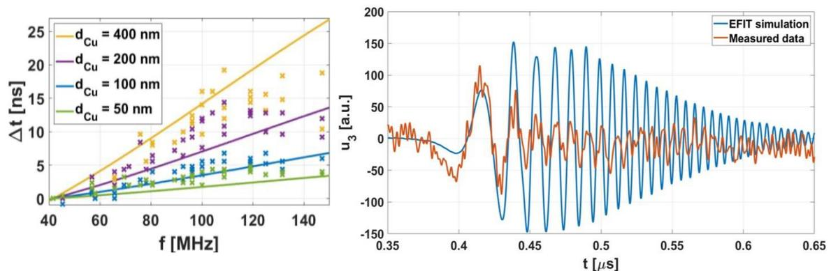
**Fig. 2.** Left: Comparison between extracted (crosses) and calculated (solid lines) dispersion behaviour of SAWs in multilayer samples with different inclusions.
