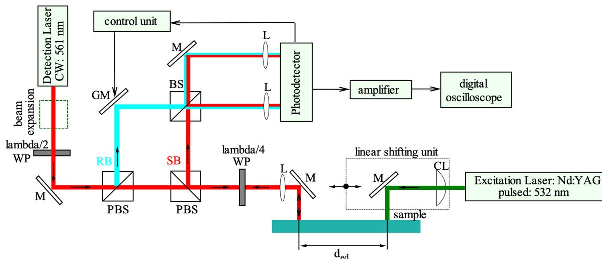
Fig. 1. LUS setup optimized in the detection of surface acoustic waves
