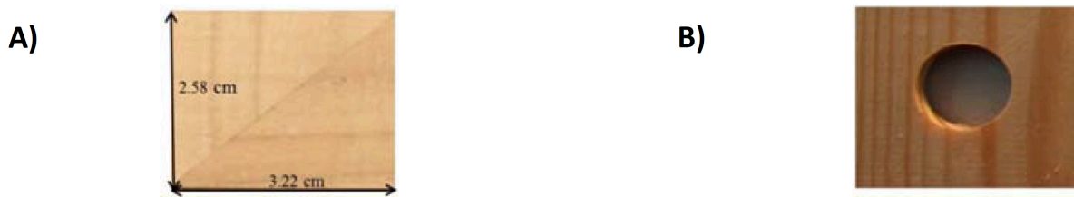
Fig. 1. (A) The irradiated mahogany veneer front layer of the marquetry sample. (B) The pine layer of the art sample with a 14-mm diameter drilled through-hole in the pine layer only.
