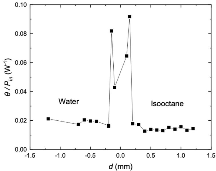
**Fig. 1.** Parameter  $\theta$  normalized to the pump beam power used for each measurement, as a function of the distance ( $d$ ) perpendicular to the interface, which is located at  $d = 0.0$  mm.
