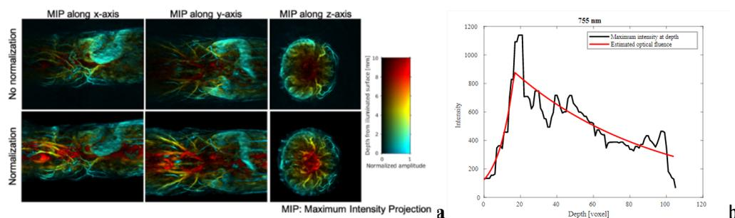
**Figure 3.** (a) Maximum intensity projections of 3D full view optoacoustic images obtained at the wavelength of 757 nm of a mouse body prior and after the optical fluence normalization on the surface and through the depth of the mouse; (b) Background absorbed optical energy measured from the experimental optoacoustic image acquired at 757 nm using an array of ultrawide-band ultrasonic transducers.
