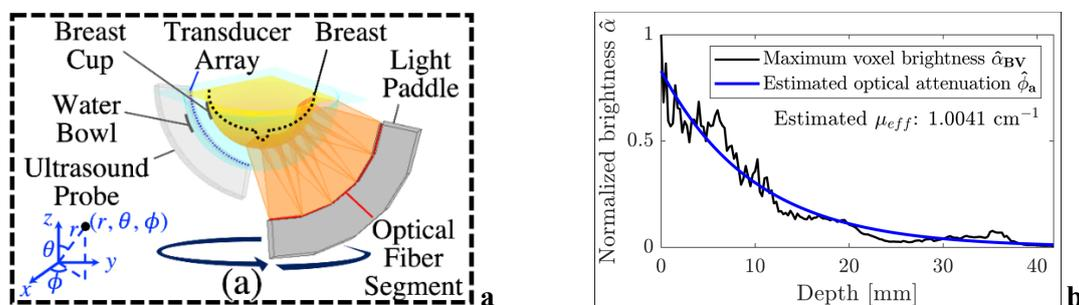
**Figure 1.** (a) Schematic diagram of the laser illumination and acoustic detection implemented in the 3D full view optoacoustic imaging system designed for detection of breast cancer. (b) Typical optical attenuation curve measured experimentally from a 3D optoacoustic image acquired using an array of ultrawide-band ultrasonic transducers from breast
