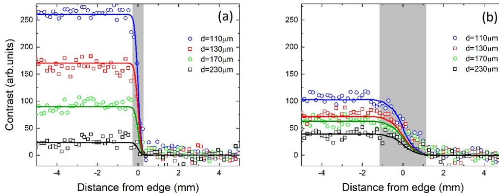
**Fig. 3.** Experimental (symbols) and theoretical (lines) contrast profiles across the inked edge areas recorded at two different delays:  $t=0.06s$  (a) and  $t=0.93s$  (b). The corresponding distortion indexes are  $\Delta=0.56$  mm (a) and  $\Delta=2.30$  mm (b), respectively.
