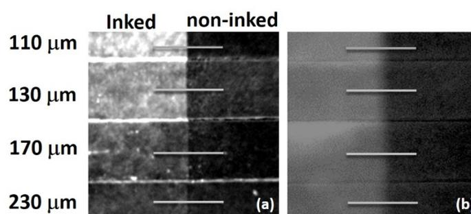
**Fig. 2.** Thermograms of the edge of the inked areas buried at different depths, recorded at (a)  $t=0.06\text{s}$  and (b)  $t=0.93\text{s}$  delays.
