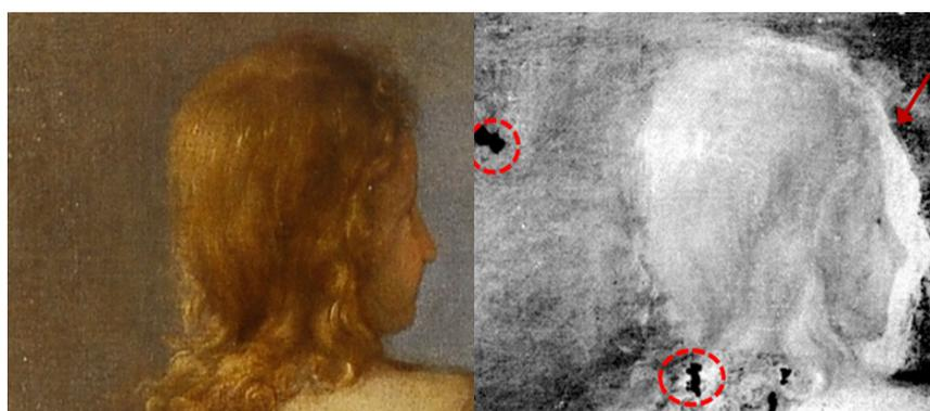
**Fig. 1.** Photo (left) and thermogram (right) of a painting revealing some *pentimenti* (arrow) and restorations (circles) beneath the surface [6].
