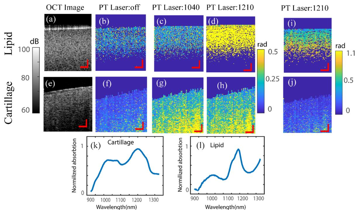
**Fig. 3.** (a) OCT image and (b-d) PT-OCT images of lipid, and (e) OCT image and (f-h) PT-OCT images of collagen samples, absorption spectrum of (k) lipid (l) collagen, and PT-OCT images of (i) lipid and (j) collagen with wider color bar.
