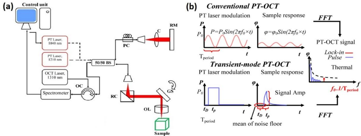
**Fig. 1.** Schematic of (a) experimental PT-OCT system; (b) laser modulation and sample responses in conventional PT-OCT and transient-mode PT-OCT.
